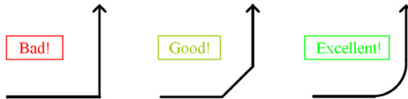
Figure 5-12: Examples of Turns in Trace Routing
